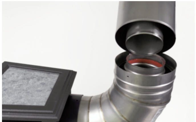
The next section of SC pipe inserts with the male end down into the gasketed female end.
